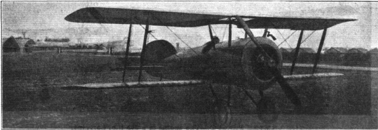
THE VICKERS F.B. 19. —This was really a development of the “Barnwell Bullet,” and has a 110 h.p. Clerget engine
